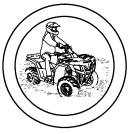
Wet brakes may have reduced stopping ability. Always test the brakes after leaving water. If necessary, apply them several times to let friction dry out the pads.
